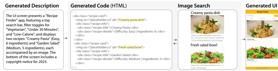
Fig. 3: An example of a generated UI description with the corresponding generated code and generated UI. In the Production phase, our pipeline extracts alternative text and placeholder image links and uses Bing Search API or DALL·E to get a link or image to replace the placeholder.
